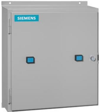
Duplex starter w/o alternator, Size 1, Three phase full voltage, Solid-state overload relay, OLR amp range 0.25-1A, 380-440/440-480V 50/60Hz coil, Non-combination type, Enc NEMA type 4 painted steel, Water/dust tight for outdoors
