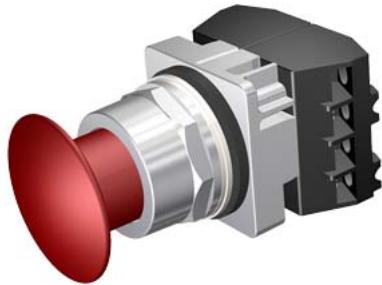
30mm Command/52, Chrome Finish Heavy Duty, Watertight/Oiltight Complete Metal Unit Push-Pull Operator Non-Illuminated Mushroom Head Cap Small 1.73" (44 mm) Metal, Anodized Red 3 Position Momentary 1 N.C.+1 N.C. Extra Late Break Heavy Duty Contacts, A600/P600 UL Listed, CSA Certified NEMA 1,3,3R,4,4X,12,13 & Automotive Standards
