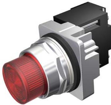
30mm Command/52, Chrome Finish Heavy Duty, Watertight/Oiltight Complete Metal Unit Illuminated Indicator Light Full Voltage type, 120V AC/DC LED Lamp, BA9s Plastic Lens, Red UL Listed, CSA Certified NEMA 1,3,3R,4,4X,12,13 & Automotive Standards
