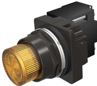
30mm BlackMax, Epoxy Coated Corrosion Resistant Complete Metal Unit Illuminated Indicator Light Transformer type, 480V AC Super Bright LED Lamp, BA9s Plastic Lens, Amber UL Listed, CSA Certified NEMA 1,3,3R,4,4X,12,13 & Automotive Standards
