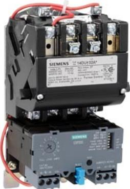
Non-reversing motor starter Size 2 Three phase full voltage Solid-state overload relay OLRelay amp range 13-52a 110VAC 50HZ / 120VAC 60HZ coil Combination type No enclosure
