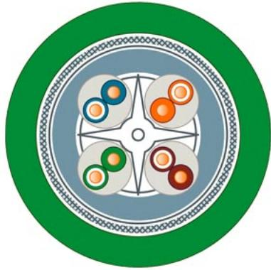
IE FC TP Standard Cable GP 4x2 (AWG 24, Type C)
