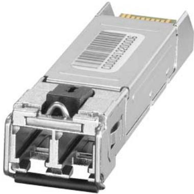
SCALANCE X accessory; plug-in transceiver SFP992-1LD; 1x 1000 Mbit/s LC port, optical; single-mode optical up to max. 10 km 1 pack = 10 units.
