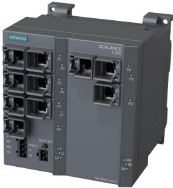
SCALANCE X310, managed plus IE switch, 3x 10/100/1000 Mbit/ and 7x 10/100 Mbit/s RJ45 ports LED diagnostics, error signaling Contact with select/set pushbutton, PROFINET IO device, network management, Integrated redundancy manager, office features (RSTP, VLAN, IGMP,..) C-plug in scope of supply.
