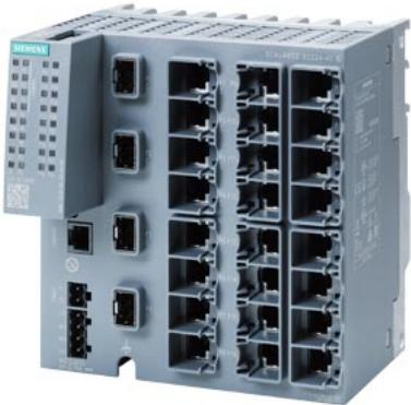
SCALANCE XC224-4C G manageable Layer 2 IE switch; IEC 62443-4-2 certified; Full gigabit; 20x 10/100/1000 Mbps RJ45 ports; 4x 1000 Mbps combo ports (either 1000 Mbps/ SFPs or 10/100/1000 Mbps RJ45 ports can be used); 1x console port; diagnostics LED; redundant power supply; temperature range -40 °C to +70 °C; assembly: DIN rail/S7 mounting rail/wall; redundancy functions; office features (RSTP, VLAN,...); PROFINET IO device; Ethernet/IP-compliant; C-PLUG slot; IEEE 1588v2 PTP
