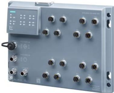
SCALANCE XP216PoE EEC, managed IE switch, with railway approval IEC 62443-4-2 certified; (EN 50155, EN45545); 12x 10/100 Mbit/s M12 ports, 4x 10/100/1000 Mbit/s M12 ports IP65, LED diagnostics, error signaling contact, redundant power supply, PROFINET IO device, network management, can be operated in redundant ring, incl. dust caps, including electronic manual on CD-ROM, C-PLUG optional.
