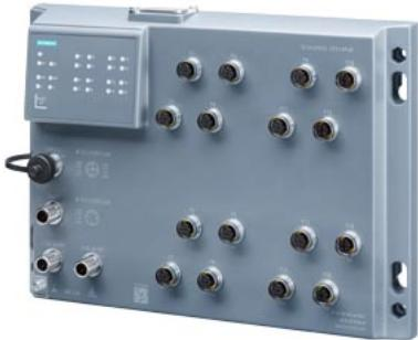
SCALANCE XP216 (EIP), managed IE switch, 12x 10/100 Mbit/s IEC 62443-4-2 certified; M12 ports, 4x 10/100/1000 Mbit/s M12 ports IP65, LED diagnostics, error signaling contact, redundant power supply, Ethernet/IP, network management, including dust caps, including electronic manual on CD-ROM, C-PLUG optional.
