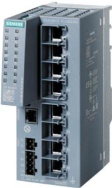
SCALANCE XC208G EEC manageable Layer 2 IE switch; IEC 62443-4-2 certified; 8x 10/100/1000 Mbit/s RJ45 ports; 1x console port; diagnostics LED; redundant power supply; with painted printed-circuit boards; NAMUR NE21-compliant; temperature range -40 °C to +70 °C; assembly: DIN rail/S7 mounting rail/wall; redundancy functions; Office features (RSTP, VLAN,...); PROFINET IO device; Ethernet/IP-compliant; C-plug slot;
