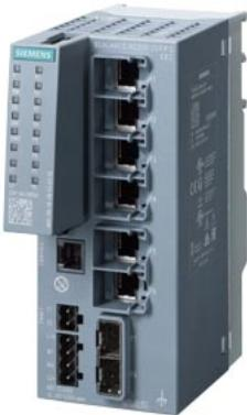
SCALANCE XC206-2SFP G EEC manageable Layer 2 IE switch; IEC 62443-4-2 certified; 6x 10/100/1000 Mbit/s RJ45 ports; 2x 1000 Mbit/s SFP; 1x console port; diagnostics LED; redundant power supply; with painted printed-circuit boards; NAMUR NE21-compliant; temperature range -40 °C to +70 °C; assembly: DIN rail/S7 mounting rail/wall; redundancy functions; office features (RSTP, VLAN,...); PROFINET IO device; Ethernet/IP-compliant; C-PLUG slot;
