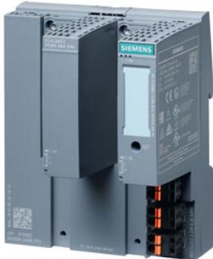
SCALANCE XF204-2BA DNA managed IE Y-switch, IEC 62443-4-2 certified; 4 x 10/100 Mbit/s, 2 x BusAdapter interface, error signaling contact, set pushbutton, redundant 24 V DC power supply, PROFINET device, extended temperature range -40 °C...+70 °C, conformal coating, with electr. manual on DVD, C-PLUG optional, supplied without BusAdapter
