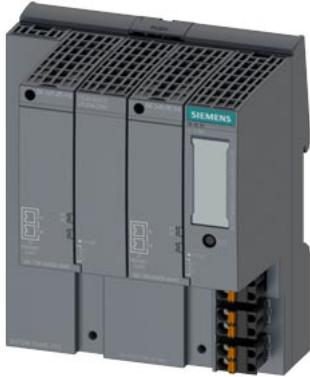
SCALANCE XF204 DNA managed IE Y-switch, IEC 62443-4-2 certified; two BusAdapters BA 2xRJ45 HA 4 x 10/100 Mbps, 2 x BusAdapter interface, error signaling contact, set pushbutton, redundant 24 V DC power supply, PROFINET device, extended temperature range -40 °C...+70 °C, conformal coating, with electronic manual on DVD, C-PLUG optional, delivery with BusAdapter.
