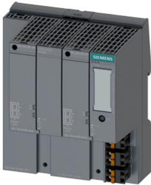
SCALANCE XF204 managed two BusAdapters BA 2xRJ45 HA IEC 62443-4-2 certified; IE switch, 4 x 10/100 Mbps, 2 x BusAdapter interface, error signaling contact, set pushbutton, redundant 24 V DC power supply, PROFINET device, extended temperature range -40 °C...+70 °C, conformal coating, with electronic manual on DVD, C-PLUG optional, delivery with BusAdapter. 6DL1193-6AR00-0AA0
