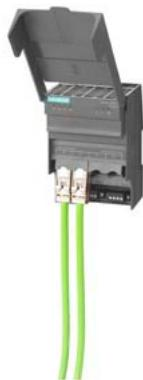
SCALANCE XF204, flat, Managed IE switch, 4x 10/100 Mbit/s RJ45 ports, Error signaling contact with set pushbutton, Redundant power supply, PROFINET IO device network management, Redundancy Manager integrated, incl. electron. manual on CD-ROM, C-plug optional.
