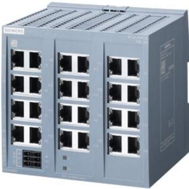
SCALANCE XB124 unmanaged IE switch, 24x 10/100 Mbit/s RJ45 ports; for setting up small star and line topologies; LED diagnostics, IP20, Redundant power supply, 24 V AC/DC Manual available as a download .
