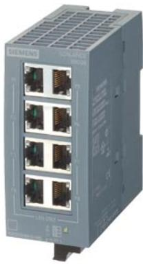
SCALANCE XB008 Unmanaged Industrial Ethernet Switch for 10/100 Mbit/s; for setting up small star and line topologies; LED diagnostics, IP20, 24 V AC/DC power supply, with 8x 10/100 Mbit/s twisted pair ports with RJ45 sockets; Manual available as a download .
