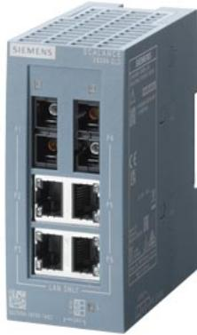
SCALANCE XB004-2LD unmanaged Industrial Ethernet Switch for 10/100 Mbit/s; for setting up small star and line topologies; LED diagnostics, IP20, 24 V AC/DC power supply, with 4x 10/100 Mbit/s twisted pair ports with RJ45 sockets; 2 x 100 Mbit/s single-mode glass fiber-optic cable port with SC socket; manual available as a download .
