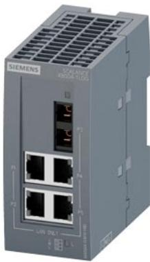
SCALANCE XB004-1LDG unmanaged Industrial Ethernet Switch for 10/100/1000 Mbit/s; for setting up small star and line topologies; LED diagnostics, IP20, 24 V DC power supply, with 4x 10/100/1000 Mbit/s RJ45 Ports electrical and 1 x 1000 Mbit/s SC-port optical (single-mode, glass), up to max. 10 km Manual available as a download .
