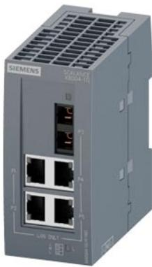
SCALANCE XB004-1G unmanaged Industrial Ethernet Switch for 10/100/1000 Mbit/s; for setting up small star and line topologies; LED diagnostics, IP20, 24 V DC power supply, with 4x 10/100/1000 Mbit/s RJ45 ports electrical and 1 x 1000 Mbit/s SC-port optical (multimode, glass), up to max. 750 m Manual available as a download .
