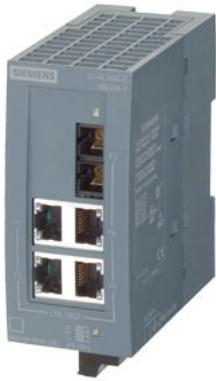
SCALANCE XB004-1LD unmanaged Industrial Ethernet Switch for 10/100 Mbit/s; for setting up small star and line topologies; LED diagnostics, IP20, 24 V AC/DC power supply, with 4x 10/100 Mbit/s twisted pair ports with RJ45 sockets; 1 x 100 Mbit/s single-mode glass fiber-optic cable port with SC socket; manual available as a download .
