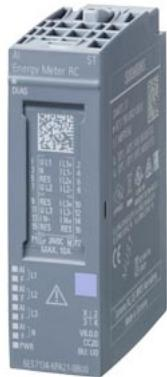
SIMATIC ET 200SP, analog input module, AI Energy Meter RC ST, for Rogowski coils or current/voltage transformer 333 mV, suitable for BU type U0, channel diagnostics
