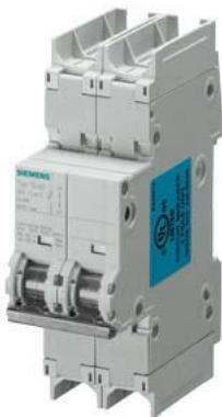
Miniature circuit breaker 240 V 14kA, 2-pole, D, 5 A, D=70 mm according to UL 489
