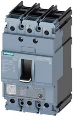
circuit breaker 3VA5 UL Frame 125 breaking capacity class H 65 kA @ 480 V 3-pole, line protection TM230, FTAM,  $I_n=125$  A overload protection  $I_r=125$  A permanently set short-circuit protection  $I_s=5\ldots 10 \times I_n$  UL 489 SB (naval), 50 degrees Celsius cable connection on two sides
