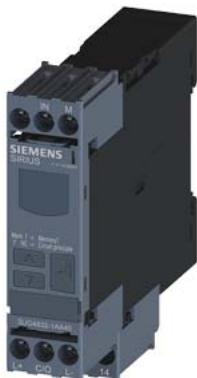
!!! product phase-out !!! the preferred successor is 3UG5842-1AA40 digital monitoring relay voltage monitoring, 22.5 mm for IO-Link 10...600 V AC/DC overvoltage and undervoltage hysteresis 0.1 to 300 V ON-delay time tripping delay time 1 changeover contact, screw terminal
