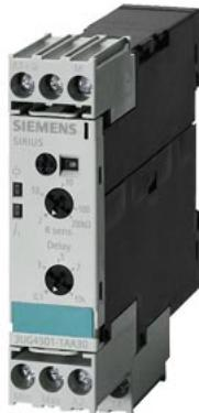
!!! product phase-out !!! the preferred successor is 3UG5501-1AW30 analog monitoring relay level monitoring resistance monitoring from 2 to 200 kohm overshoot and undershoot supply voltage 24 V AC/DC 50 to 60 Hz DC and AC without electrical isolation to measuring circuit 2-step or 1-step control tripping delay 0.5 to 10 s 1 changeover contact screw terminal
