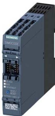
basic device SIMOCODE pro S, PROFIBUS DP interface 1.5 Mbps, 4 I/2 O freely configurable, Us: 24 V DC, input for thermistor connection monostable relay outputs, expandable by a multifunction module
