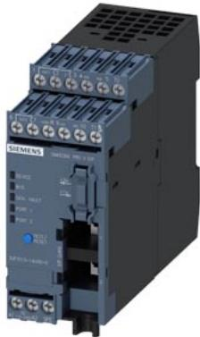
basic device SIMOCODE pro V EIP, EtherNet/IP, media redundancy, DLR (max. 20 participants) web server, transfer rate 100 Mbps, 2 x bus connection via RJ45, 4 I/3 O freely configurable, Us: 110...240 V AC/DC, input for thermistor connection monostable relay outputs, expandable by expansion modules
