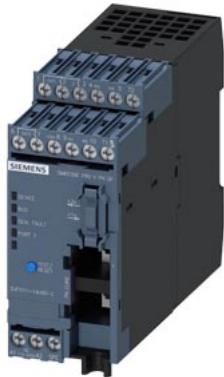
basic device SIMOCODE pro V PN GP , Ethernet/PROFINET IO, PN system redundancy, OPC UA server, web server, transfer rate 100 Mbps, 1 x bus connection via RJ45, 4 I/3 O freely configurable, Us: 110..240 V AC/DC, input for thermistor connection monostable relay outputs, expandable by 1 expansion module(DM, TM, EM)
