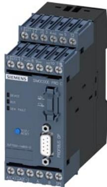
basic device SIMOCODE pro C, PROFIBUS DP interface 12 Mbps, RS-485, 4 I/O freely configurable, Us: 24 V DC, input for thermistor connection monostable relay outputs
