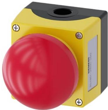
Enclosure for command devices 22 mm, round, Enclosure material metal, Enclosure top part yellow, 1 control point metal, Control point in center, A=EMERGENCY STOP palm pushbutton, red, positive latching, pull-to-unlatch mechanism, 1 NC, 1 NO, screw terminal, Floor mounting
