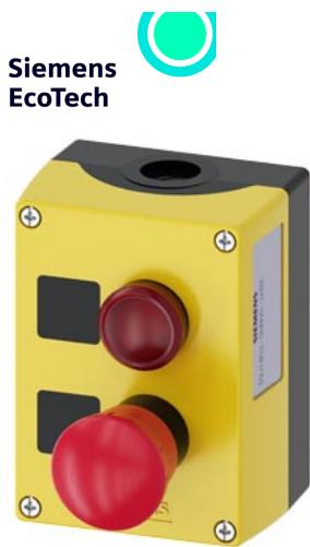
enclosure for command devices, 22 mm, round, enclosure material plastic, enclosure top part yellow, 2 command points plastic, B=indicator light red, LED 24 V, screw terminal, LED 24 V, screw terminal, label without inscription, A=EMERGENCY STOP 40 mm rotate-to-unlatch, label without inscription, 1 NO, 1 NC, 1 NC, screw terminal, base mounting, 1x M20 each on top and bottom, labels enclosed
