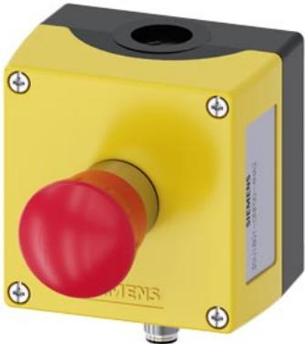
Enclosure for command devices, 22 mm, round, enclosure material plastic, enclosure top part yellow, 1 control point, plastic, A=EMERGENCY STOP mushroom pushbutton red, 40 mm, rotate-to-unlatch, 1 NO, 1 NC, spring-type terminal, floor mounting, wired, without label, at bottom M12 connector 4-pole
