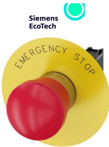
EMERGENCY STOP mushroom pushbutton, 22 mm, round, metal, shiny, red, 40 mm, positive latching, acc. to EN ISO 13850, pull-to-unlatch mechanism, with yellow backing plate, inscription: EMERGENCY STOP, with holder, 1 NC, screw terminal
