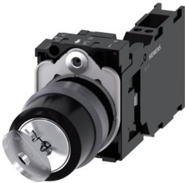
RONIS keyswitch, 22 mm, round, plastic with metal front ring, Lock number SB30, with 2 keys, 2 switch positions O-I, latching, 10:30/1:30 o'clock, key removal O+I, with holder, 1 NO+1 NC, spring-type terminal, possible special locks: SB31, 421, 455
