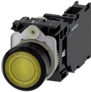
Illuminated pushbutton, 22 mm, round, plastic, yellow, pushbutton, flat, momentary contact type, with holder, 1 NO+1 NC, LED module with integrated LED 110 V AC, spring-type terminal, with laser labeling, upper case and lower case, always upper case at beginning of line
