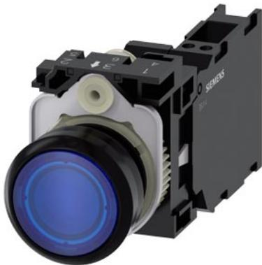
Illuminated pushbutton, 22 mm, round, plastic, blue, pushbutton, flat, momentary contact type, with holder, 1 NO+1 NC, LED module with integrated LED 24 V AC/DC, Spring-type terminal
