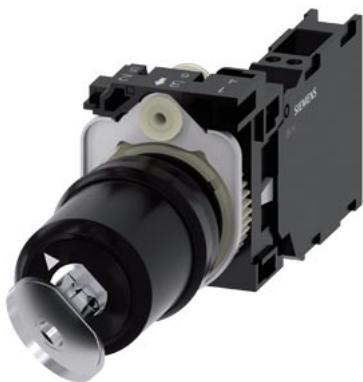
Siemens keyswitch, C, 22 mm, round, plastic, lock number S-10-CG, with 2 keys, 2 switch positions O-I, latching, 10:30h/13:30h, key removal O+I, with holder, 1 NO+1 NC, spring-loaded terminal
