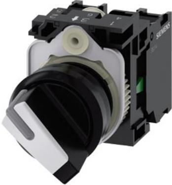
Selector switch, illuminable, 22 mm, round, plastic, white, selector switch, short, 2 switch positions O-I, latching, 10:30h/13:30h, with holder, 1 NO, 1 NC, screw terminal
