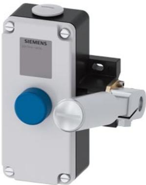
Conveyor belt unbalance tracker Metal enclosure, 2 x M25 x 1.5 2 NO+2 NC, with latching according to EN ISO 13850 Pushbutton release
