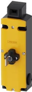
safety position switch with guard lock locking force 2600 N 5 approach directions spring-locked auxiliary release with lock magnet voltage 24 V DC monitoring actuator 2 NC/1 NO monitoring magnet 2 NC/1 NO, supplied without actuator, actuator 3SE5000-0AV0, please order separately
