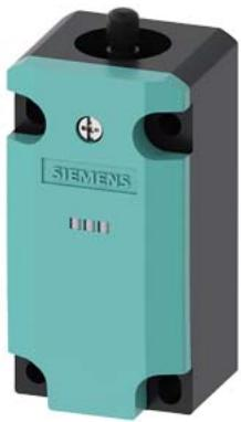
Basic switch for position switch 3SE51 Metal enclosure 40 mm according to EN 50041 Device connection 1x (M20 x 1.5) with 2 LEDs, 230 V AC yellow/green 1 NO/2 NC quick action contacts without actuator head
