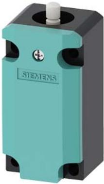
Position switch Basic switch Metal, 40 mm, according to EN 50041 Increased corrosion protection Device connection 1 x (M20 x 1.5) 1 NO/2 NC slow-action contacts functional at -40 °C Shock and vibration test according to EN 61373, Category 1B
