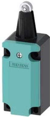
Position switch Metal enclosure 40 mm according to EN 50041 Roller plunger with Stainless steel roller 13 mm, 3 mm overtravel, 1 NO/1 NC quick action contacts, Device connection 1x (M20 x 1.5), actuating/restoring force 30 N only available as complete unit
