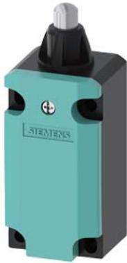
Position switch Metal enclosure 40 mm according to EN 50041 Device connection 1x (M20 x 1.5) 1 NO/1 NC quick action contacts with rounded plunger Stainless steel plunger with 3 mm Overtravel functional at -40 °C Shock and vibration test according to EN 61373, Category 1B
