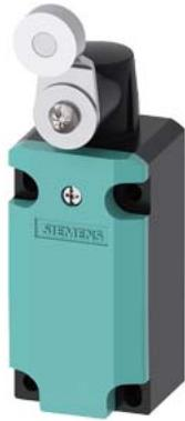
Position switch Metal enclosure 40 mm according to EN 50041 Device connection 1x (M20 x 1.5) 1 NO/1 NC slow-action contacts Rotary actuator right/left adjustable, Metal lever 27 mm long and stainless steel roller 19 mm
