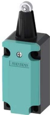
Position switch Metal enclosure 40 mm according to EN 50041 Device connection 1x (M20 x 1.5) 1 NO/1 NC slow-action contacts Roller plunger with Stainless steel roller 13 mm
