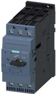
Circuit breaker size S2 for starter combination Rated current 65 A N-release 845 A screw terminal increased switching capacity
